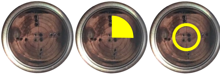
Figure 3: A photograph of the 16-segment detector in different arrangements: sector (middle), concentric circle (right)
